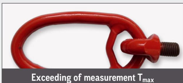
Exceeding of measurement  $T_{max}$
