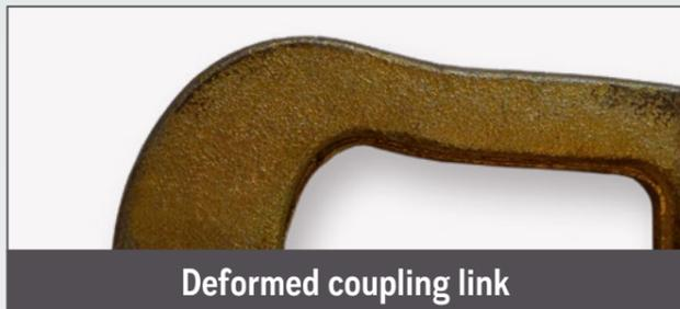
Deformed coupling link
