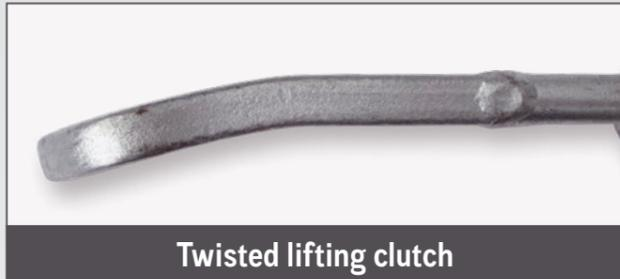
Twisted lifting clutch
