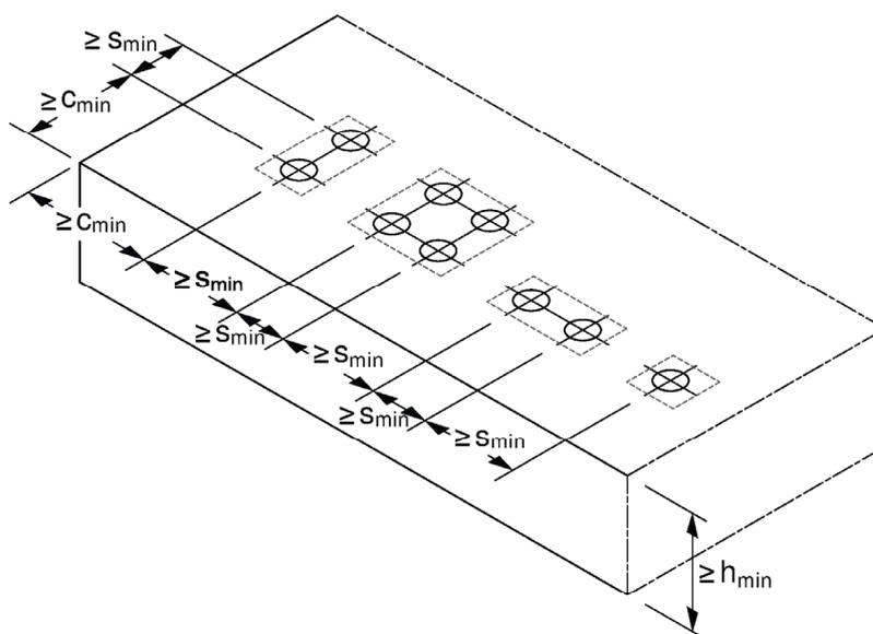
Spacing, edge distance and minimum thickness of concrete member apply also for anchors in front-side installation.
