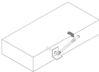
Maximum setting torques max.  $T_{inst}$  for PB Anchor
