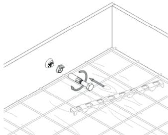
3. If required, fix supplementary reinforcement to the socket by using PHILIPP Data Clip.
