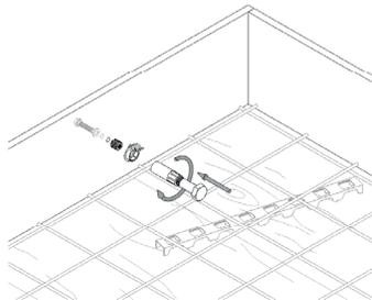
1. Put Data Clip onto the socket
