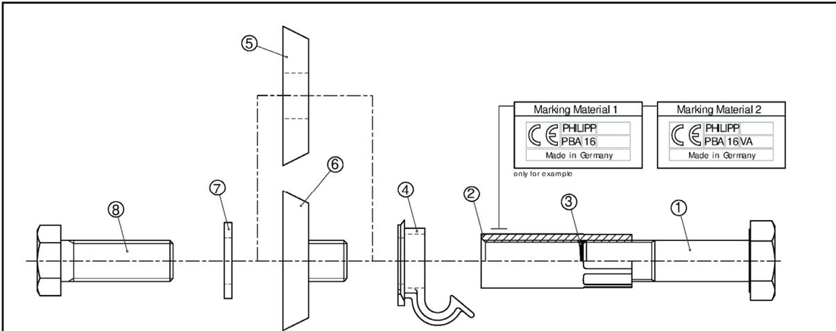
Table A3: Specification and material of the anchor and appropriate components
